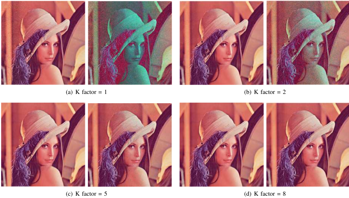
Fig. 8: Performance comparison between 2x1 Alamouti STBC and conventional 1x1 configurations over Rician fading
