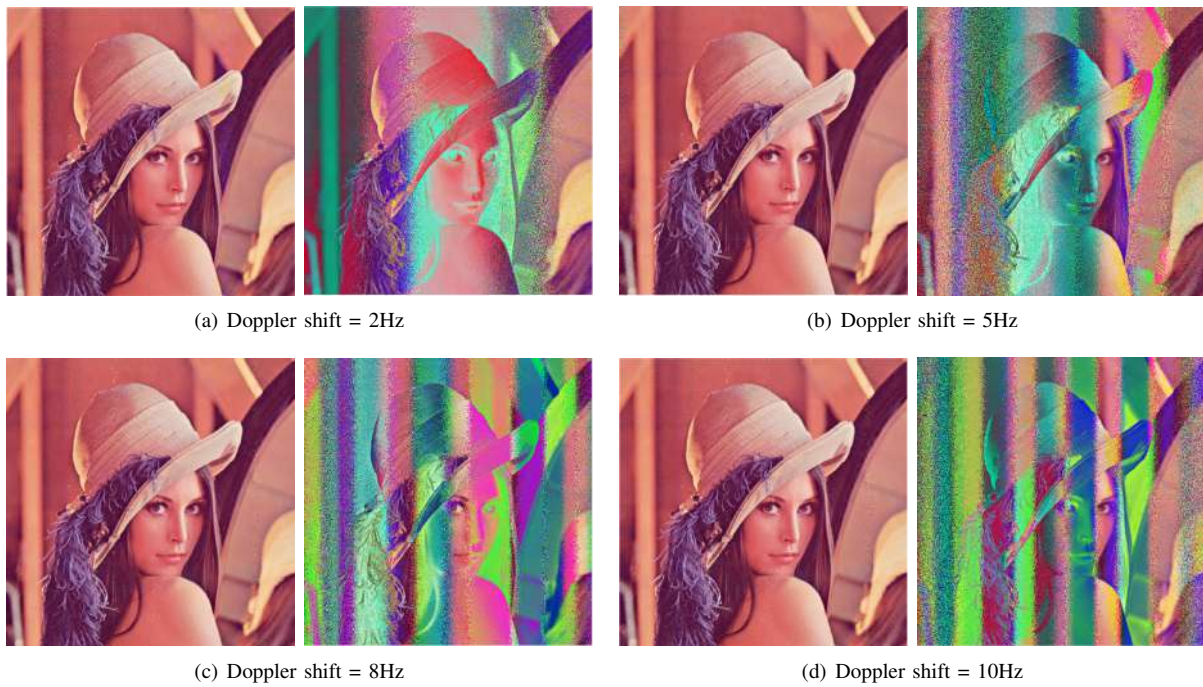
Fig. 7: Performance comparison between 2x1 Alamouti STBC and conventional 1x1 configurations over Rayleigh fading
