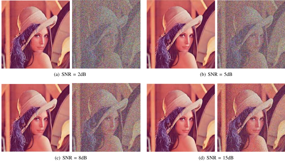
Fig. 6: Performance comparison between 2x1 Alamouti STBC and conventional 1x1 configurations over Rayleigh fading
